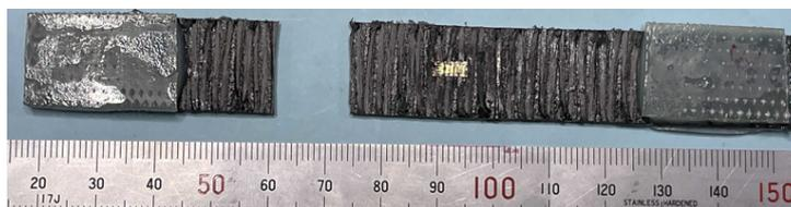
(c) 90° specimen with continuous carbon fibers.
